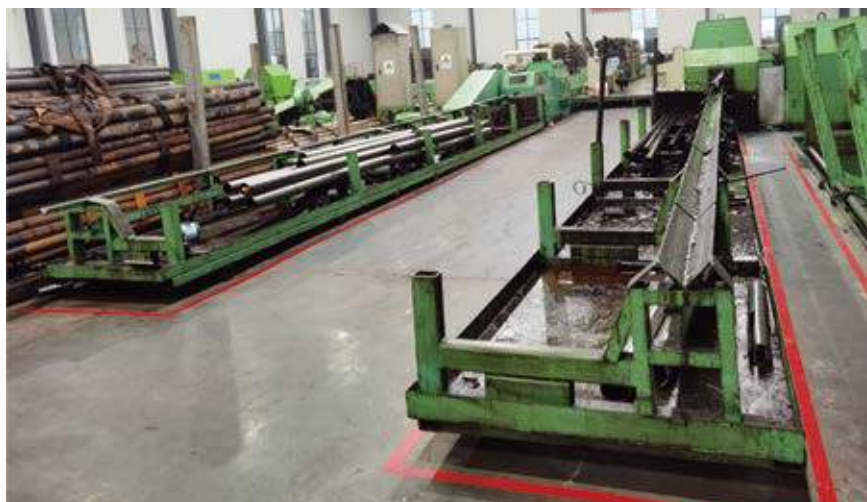
Seamless steel pipe finishing production line
