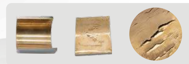
Adhesion test of bimetallic composite layer
